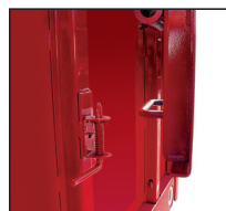
Doors open and lock to the side of the body with conveniently placed latches that can be operated from ground level.
