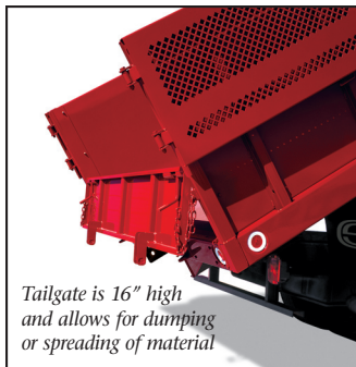
10 gauge punched hole steel double doors swing around and lock out of the way
